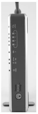
This model also includes the Cisco SES button; however, it is not labeled "Cisco". The button is yellow in color and is simply labeled "Secure Easy Setup," as shown in Figure 1.20.
