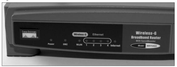
Except for the addition of SES button, version 2.0 of the WRT54GS is identical to its version 1.1 counterpart. The GS version still utilizes the Broadcom BCM4712 processor, 8 MB of Intel flash, 32 MB of Hynix DDR-SDRAM, the Broadcom BCM5325 Ethernet MAC, and the Broadcom BCM2050 wireless chipset. Table 1.13 lists the specifications of the WRT54GS, version 2.0.
