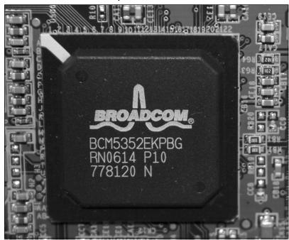
Figure 1.3 Broadcom BCM5352 Chip from a Version 1.1 WRT54GL
