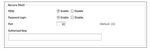
You must click **Save Settings** and then **Restart Router** before your changes will take effect. At this point, using any SSH client, you should be able to SSH to your router, as shown in previous examples. Once verified, you can disable Telnet by going to the DD-WRT Web interface, navigating to **Administration** | **Services** | **TELNET**, and choosing **Disable**, as shown in Figure 3.8.
