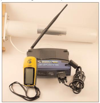
With all of these steps complete, you should be able to obtain your wardriving information off the SD card. After your wardrive, you should power off your wardriving-in-a-box WRT54G before removing the SD card from the router so that you do not corrupt the data or damage the SD card itself.
