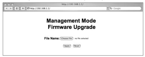
Select **Choose File**, and choose the vxworks\_killer\_g\_v06.bin file you downloaded earlier. Click **Apply**. After waiting a minute (or two), unplug your router and plug it back in. The Power light should now be flashing, indicating that the CFE is waiting for a new firmware image via TFTP. Now, you merely need to upload one using one of the TFTP methods covered earlier in this chapter. Figure 2.12 displays an example.
