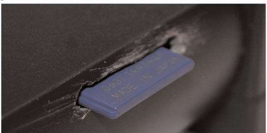
Figure 7.21 Final WRT54G SD Card External Connector
