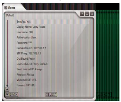
Under Windows, the configuration is a little bit different. You can find the settings under **Menu** | **SIP Account Settings**. To create a new connection click **Add**, and to modify an existing connection click **Properties**. The settings we need to define under the Account tab for our example, also reflected in Figure 4.9, are:
