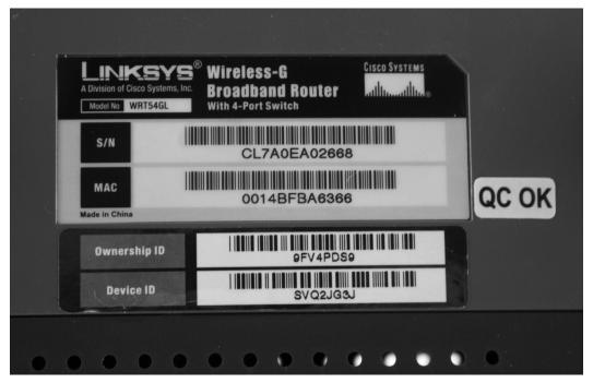
Figure 1.8 shows the "Model No" field as being "WRT54GL," which indicates the type of device. But which version of the WRT54GL are we looking at? For that information, we need to look at the first four characters in the serial number—in this case, "CL7A"—and then refer to Table 1.2.
