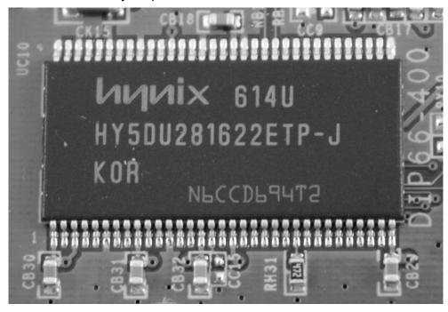
Figure 1.5 RAM Memory Chip from a Version 1.1 WRT54GL
