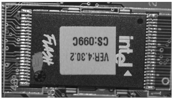
The more flash storage you have, the better, because it means you can load more software (kernel and software packages) onto the device. WRT54GS models with version numbers from 1.0 through 3.0 and the WRTSL54GS series contain the most on-board flash in the entire WRT54G family, with 8 MB.
