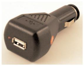
Contained within our automotive power converter is the appropriate circuitry to maintain a constant 5 volts DC at USB amperages (100 to 500 milliamps). By using the adapter and our USB cable modification, we can safely provide appropriate voltage to the WRT54G as well as isolate the router from the automotive electrical system.
